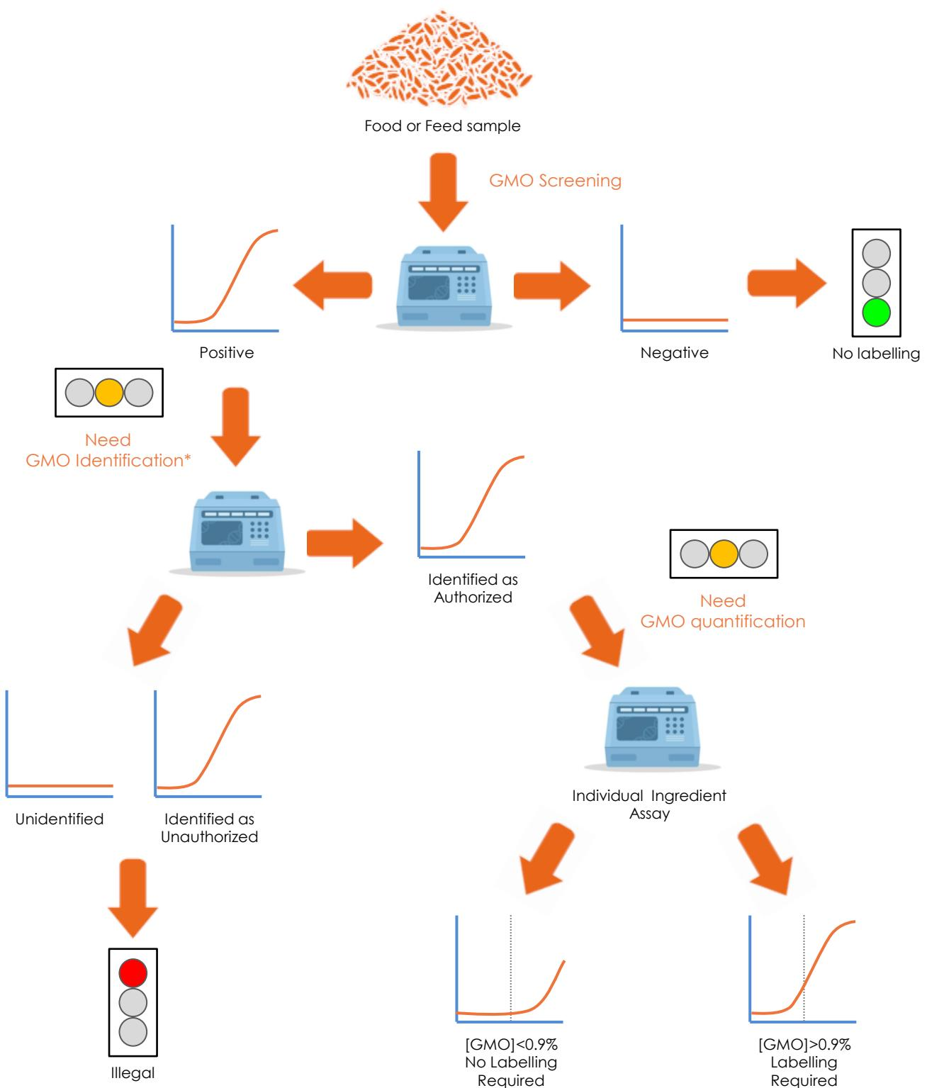
(\*) When testing complex matrices composed by more than one ingredient is fundamental to have knowledge of the different plant varieties (taxa) present in the sample in order to restrict the number of GM specific test to be performed.
